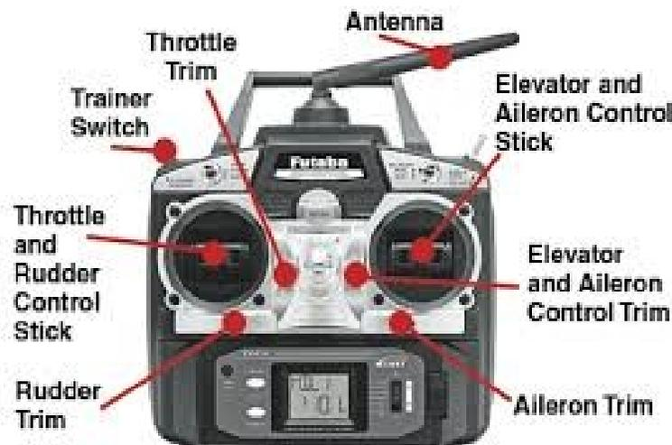
**Figure 2. Transmitter Illustration (also sometimes called radio or control box)**
